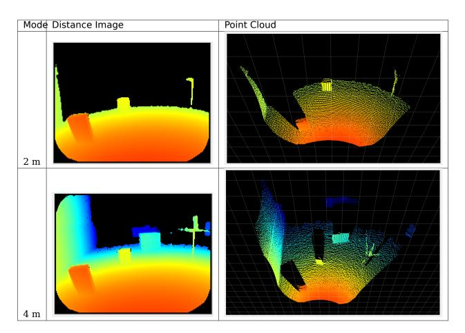
The third box, which is three meters away from the camera, is outside of the measurement range when using the two-meter mode; however it is visible when using the four-meter mode.
