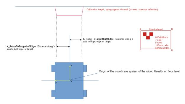
• Measure the Z\_WallToGround (line 16) and Z\_TargetToGround (line 17) as:
