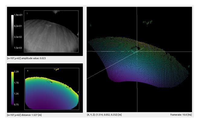
We choose a reference pixel on the side of the box. The distance measured for this pixel is  $1.527\ \mathrm{m}.$
