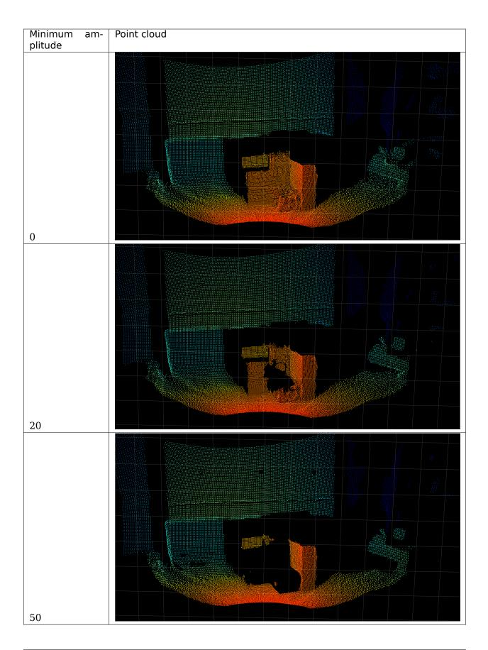
In certain cases, such as when black objects are in the field-of-view, changing the default value from 20 to zero can be beneficial because more pixels are valid, leading to a more complete point cloud. Generally speaking, lowering the amplitude leads to more ambient noise and less accuracy in the distance measurement. In this case, we encourage you to test the filters available with the O3R to mitigate the noise from black objects measurements.
