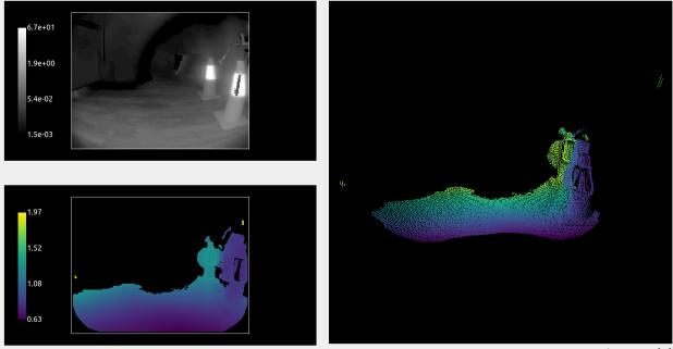
NOTE: This scene could also be handled with the amplitude threshold (diParam. excessiveCorrectionThreshAmp). This threshold follows the same concept as the distance threshold, invalidating pixels with an amplitude below the set value. Generally, setting the distance threshold suffices, but we encourage you to play with both to select the best configuration possible for your use case.
