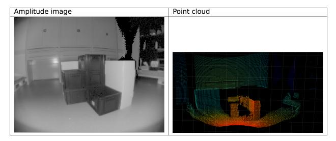
Now, let's see what happens when we change this threshold value. In the table below, we display the same scene measured with different amplitude thresholds. With a value of zero, we can compute the point cloud for the very dark areas. When we increase the threshold to 50, a large part of the point cloud is lost.
