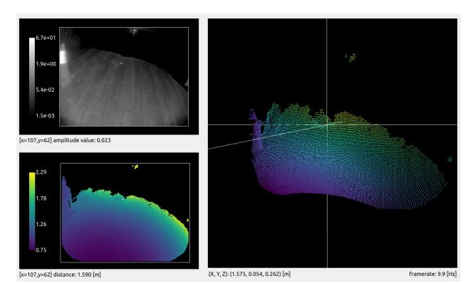
We can see that we are able to recover most of the pixels from the side of the box. However, the distance measured for the same pixel is now 1.590 m, when our reference measurement is 1.527 m. The side of the box is measured 6.3 cm off its actual position. This is acceptable because the robot will be able to drive along the reflector and still detect the presence of an obstacle.
