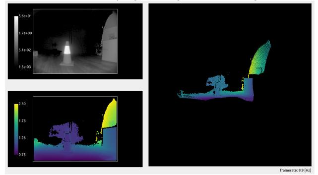
A cardboard box is positioned next to the cone, at the same distance from the camera. The halo is still there and affecting part of the background pixels. However, the measurement of the actual box is accurate and is not affected by the reflective object next to it. Stray light affects the low-signal pixels in the scene more strongly, and, in this case, it does not affect the measurement of the box, which reflects enough light.
