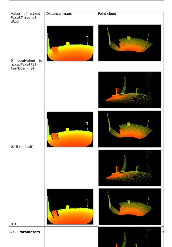
We can see that using higher values for the mixedPixelThresholdRad invalidates more pixels. We typically recommend deactivating the filter or using small values for the threshold.
