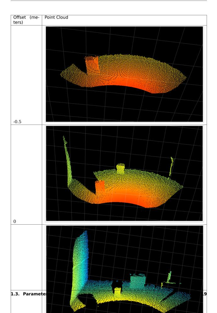
Note: In the last image where the offset is set to 2.5m, we can see that the noise is higher than in the other images. This is due to the distance to the camera, with which the noise increases, and to the fact that the most robust measurement is in the middle of the range, which is from around 3 to 4 m in the case of the last example. The ground in front of the box is outside of the robustness area.
