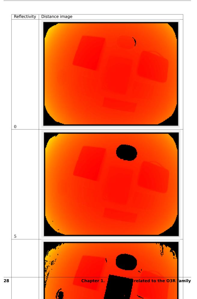
Note: In the first image, some pixels are missing from the side of the object. This area of the object does not reflect enough light, even when a low reflectivity threshold is allowed.
